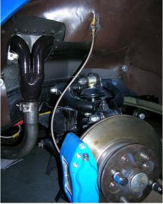
Photos: Previous page top, nearside rear showing the Hoyle IRS seen from behind - note the Sierra disc brake and drive shaft, upper and lower wishbones and alloy hub carrier – and lower, Mike's 1969 MGBGTV8. This page top, front offside showing the Hoyle front suspension with four pot caliper and vented disc. Lower photo, detail of the front suspension - note snail cam to adjust the camber. The anti-roll bar fits on the lower wishbone.
