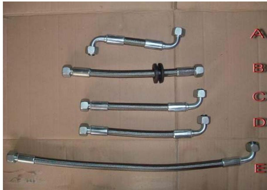
For top mounted oil coolers hoses C & E would need to be shorter, by the depth of the cooler and terminate with 90deg' elbows.
