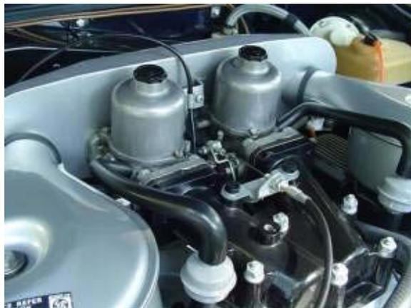
Topping up the dampers on the twin SU HIF carburetors on an MGBGTV8 is a very worthwhile simple service routine which can make driving the MGBGTV8 so much more enjoyable with a smoother pick up and acceleration and a less frisky engine at slow speeds. Enthusiasts not familiar with SU carburetors may not be aware of the benefits of regular damper topping-up or what to do, so this note is a straightforward guide.
