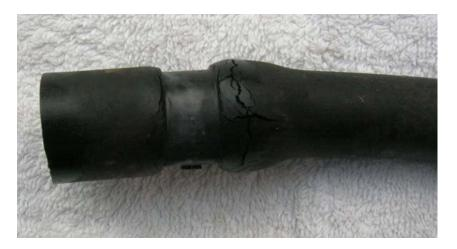
Close up of the failure of **BHH1083 heater to outlet pipe** hose from which a jet of hot coolant was escaping as liquid and steam. You can see the hose has split at a point which is just behind the engine so conditions can get very hot in that area – conditions which give a rubber hose a very hard service life.
