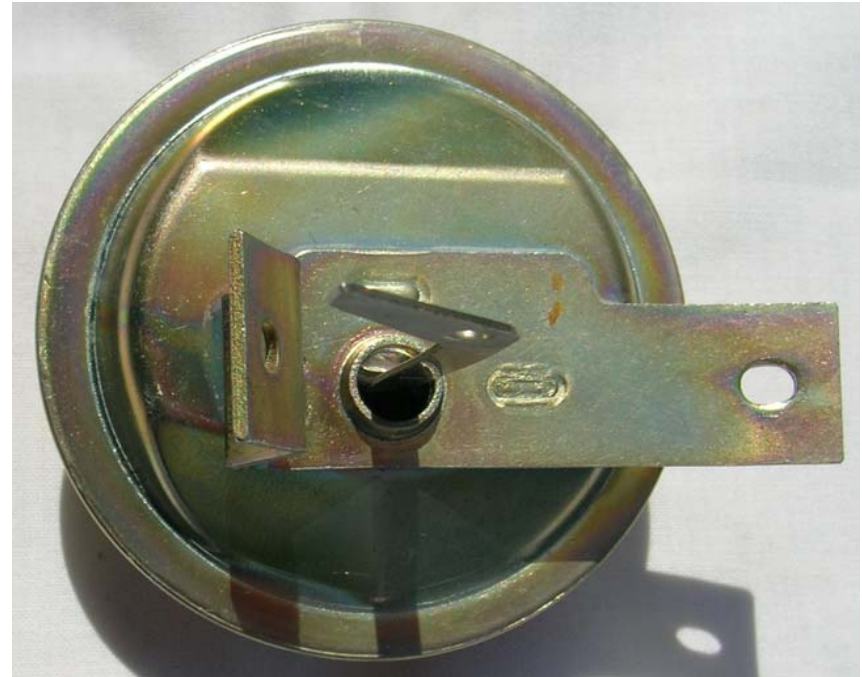
Left: connecting spout on the replacement distributor vacuum unit is in a different position to the original, which was on the tip rather than the side.
