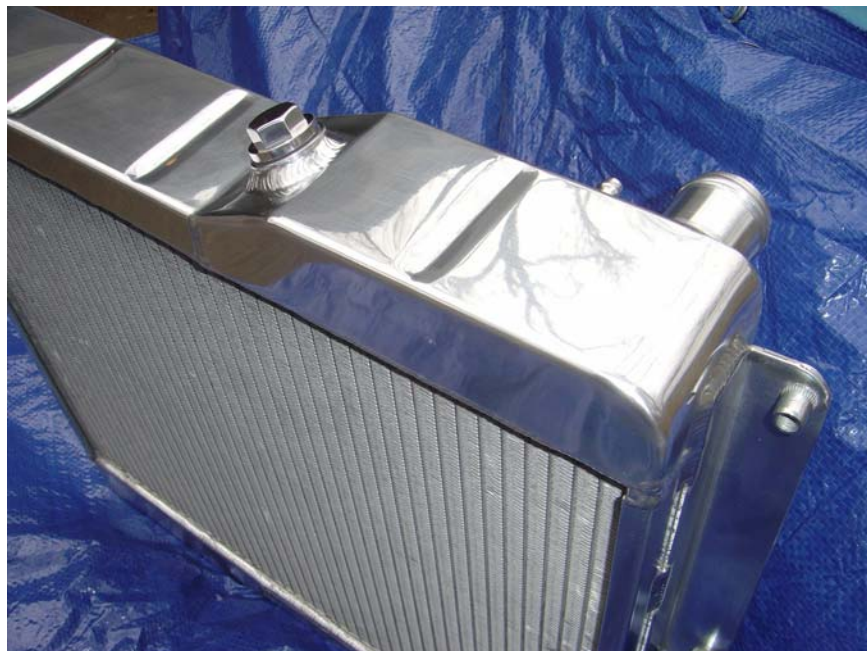
MGB V8 high efficiency alloy radiator. The supplier, Radtec, says it offers a 35% upgrade in cooling over the original radiator fitted by the Factory and they add the "fitment is as original".
