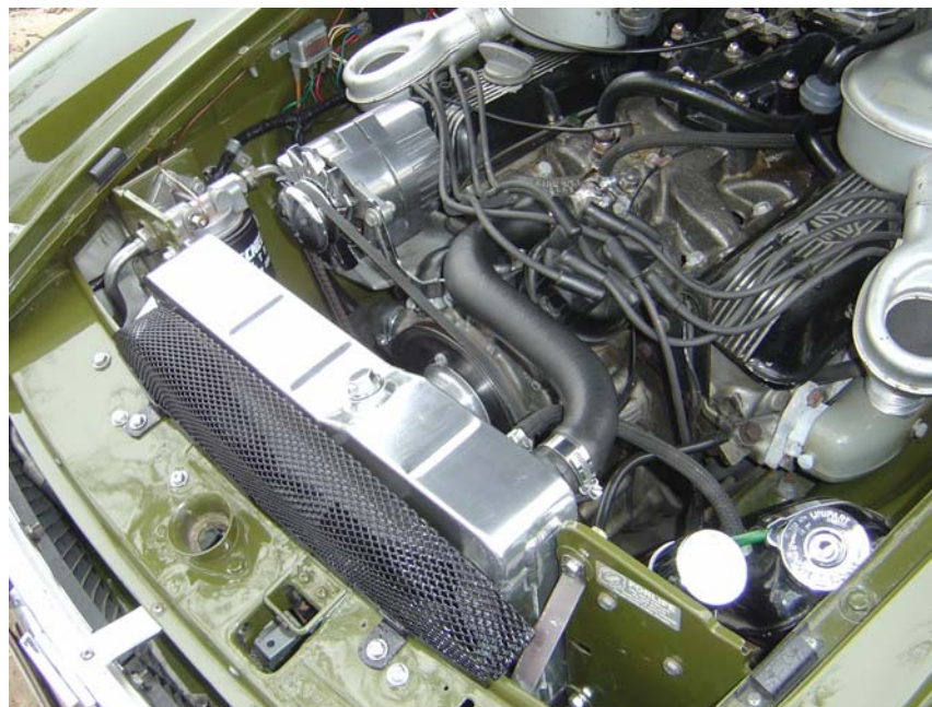
MGB V8 high efficiency alloy radiator. The supplier, Radtec, says it offers a 35% upgrade in cooling over the original radiator fitted by the Factory and they add the "fitment is as original".
