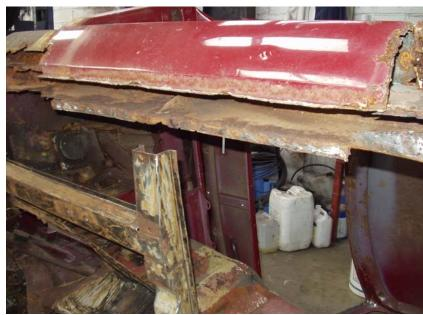
The floor has been removed from the nearside, along with the remains of the jacking point. Where it meets the inner sill, the cross-member was found not to be sound, needing a small repair at the very end.
