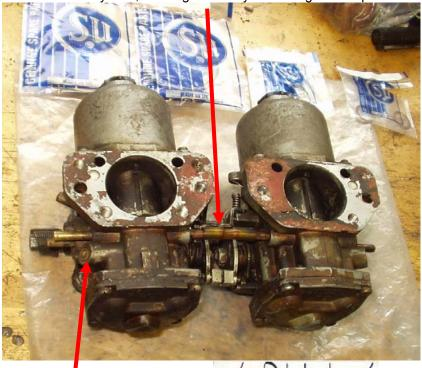
The mixture adjustment screws are still covered with tamper-proof caps. This was probably done to all new V8s before they left the Factory. After I fit new jets and needles I will have to remove these caps in order to adjust the mixture.
