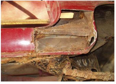
In order to insert a complete new outer sill, it is necessary to remove a small section of the rear wing. This revealed that the rear part of the sill had been cut away but not replaced when the sill was previously repaired some years ago.
