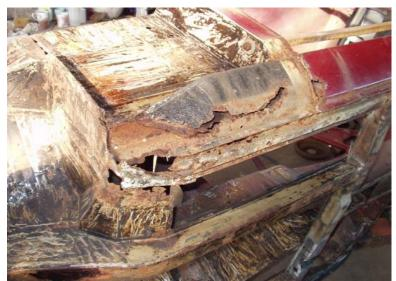
Turning my attention to the passenger side, I wondered if it would be a repeat of the driver's side. However, it had a few surprises in store. Another steel bar has been inserted across the door frame as a temporary measure, in order to preserve the rigidity of the shell, after which the floor pan has been cut out. Behind the front wing, both the sill and the castle section have corroded badly - far worse than it seemed before the wing was removed.
