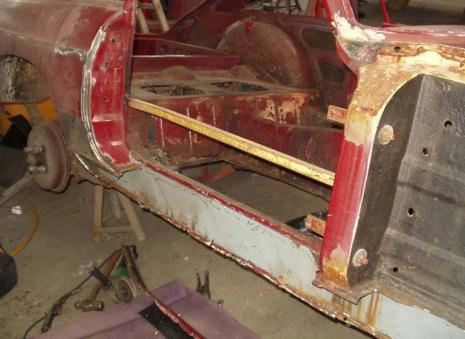
The driver's inner step sill was holed in two places, so it needed replacing. There is a repair section available that is 4 feet long and avoids the need to remove the rearmost part. However, this does require a butt weld, which would create a weak point. In order to overcome this, a strengthening plate has been welded over the join. This completes the preparation of the driver's side, prior to sand blasting.
