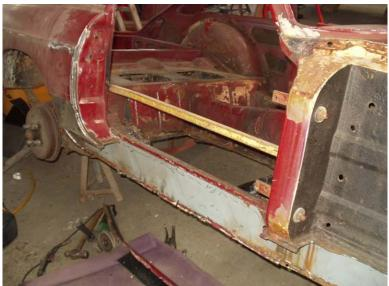
After a holiday break, work resumes on Damask 0450. The time has come to remove the outer sill on the driver's side. The floor pan has already been removed, so to prevent the shell from losing its shape a steel bar has been welded across the door frame as a temporary measure. Below is the view from inside the car . . .
