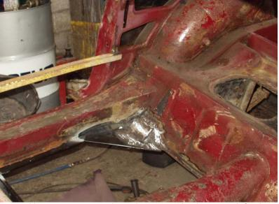
. . . and here we can see where the new spring hanger reinforcing panel has been inserted. The new floor pans will not be inserted until after the shell has been sand-blasted.
