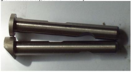
Finally, I noticed that the gear lever could not move sideways sufficiently to touch the circular gate bolted to the top of the remote unit. The gear lever is prevented from rotating by two dowel bolts, and adding one washer under the head of each bolt was all that was necessary to provide sufficient clearance for the lever to operate properly.
