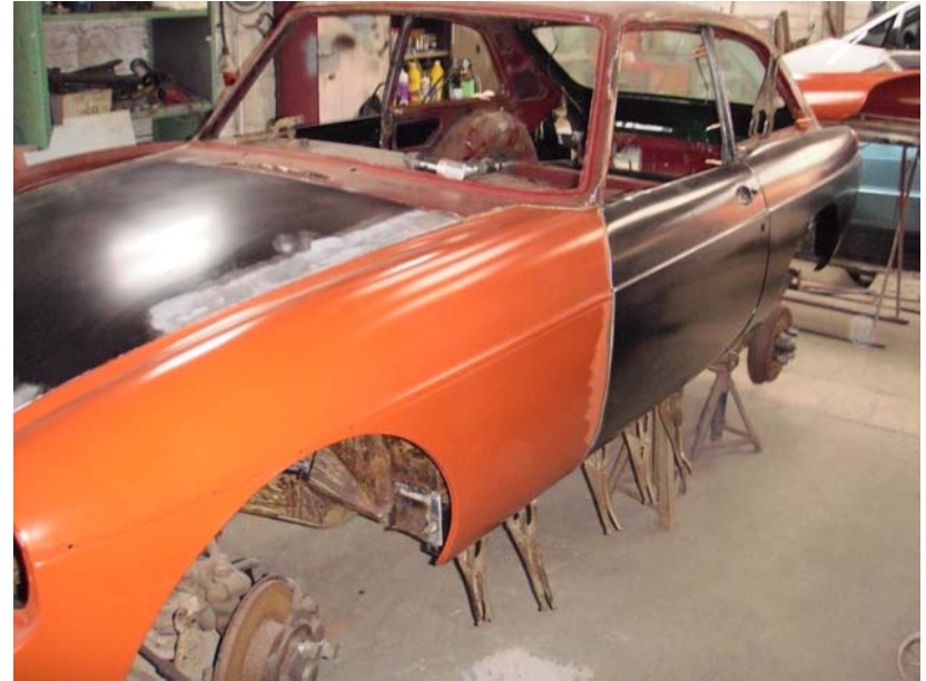
Above: all the non-structural panels (doors, wings, bonnet and tailgate) have been test-fitted and the panel gaps adjusted to suit. Below: bonnet after fettling.
