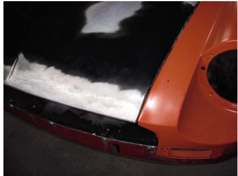
Above: all the non-structural panels (doors, wings, bonnet and tailgate) have been test-fitted and the panel gaps adjusted to suit. Below: bonnet after fettling.
