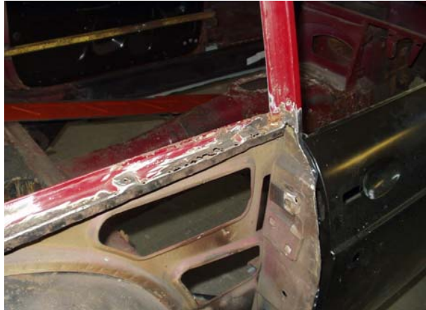
Under OSR window - the area behind the rain channel is also a common rust area, and this one proved to be no exception.
