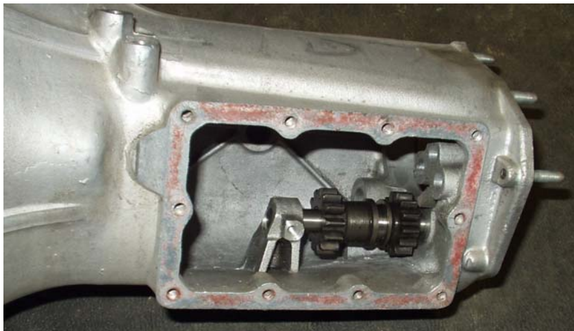
Main casing which clearly shows a weak point. Looking through the side access plate you can see the support pillar for the reverse gear shaft. Notice how it attaches to the bottom of the casing.
