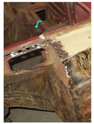
Also, at the front, the nearside 'trumpet' has been removed. This has revealed a frilly edge which would otherwise have gone unnoticed.
