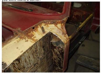
This week, the boot floor came out. Not only was it totally rusted out, but also it gave access to the rear chassis rails, which were holed in several places.
