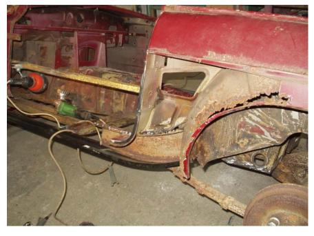
In the **second photo** you get a better view of the inner wheel arch, which will be replaced shortly. Underneath, you can just make out the new bottom fitted to one of the battery carriers. These always rust badly. I like to reposition the forward stop further forward, so that a pair of 12 volt batteries can be fitted. I use standard 063 batteries, which are very common and readily available.
