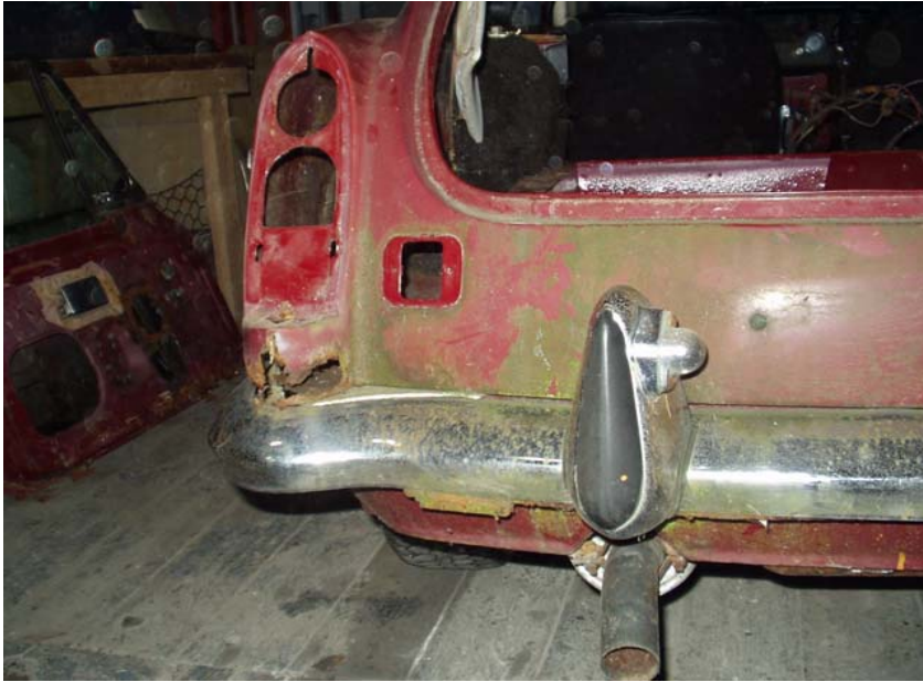
Rear nearside wing was badly rusted out around the tail lamp, particularly below the light fitting
