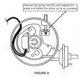
Note: the adjusting bolt is not removed, just the spring.
