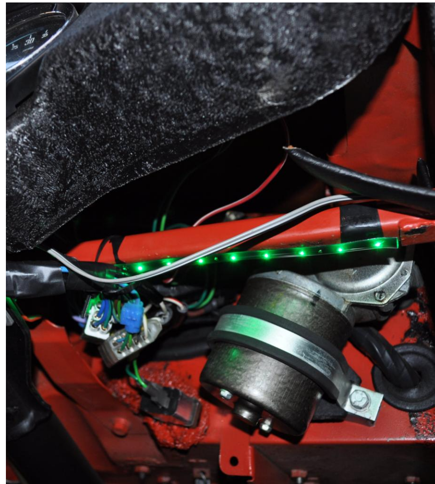
Above: lights fitted to the offside box section cross brace above the legwell
