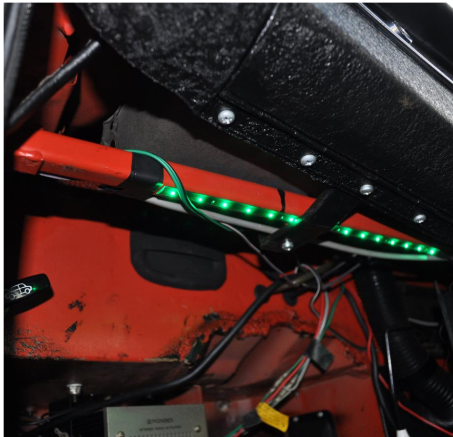
Above: lights fitted to the nearside box section cross brace above the legwell
