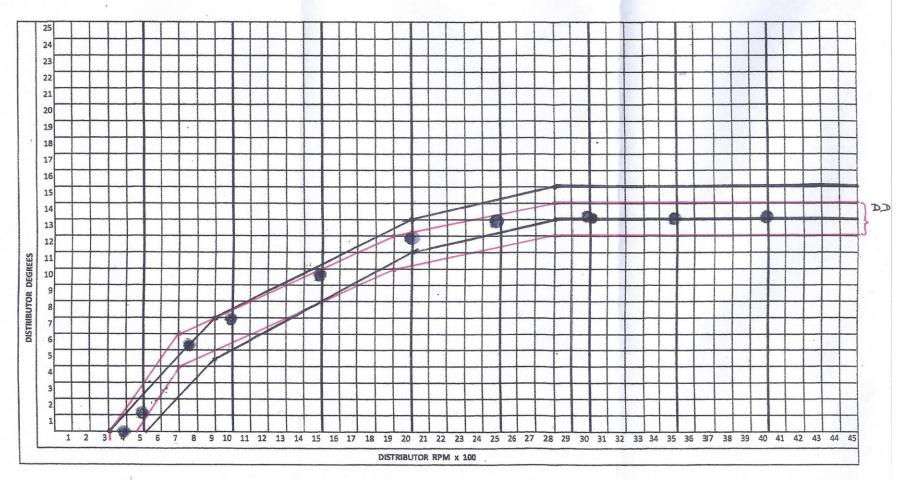
The black curves (upper and lower tolerances) are for the Lucas 35D8 41394 distributor originally fitted to the MGBGTV8 model and the red curves are for the new distributors the Distributor Doctor has available as a brand new replacement. The black dots are the measurements of a new distributor under test. Tolerances: 2%.
