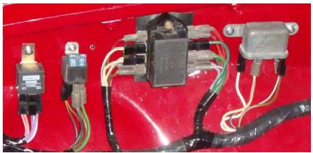
Barrie Jones reports - Damask 450 is now fully painted, and I have fitted all the wiring, brake lines, fuel line, dashboard, suspension and brakes. The top photo shows the fuel line with a Filter King fitted and the lower the wiring and relays in the engine compartment. Next step is to hoist the engine back in, with gearbox and overdrive already attached. Then all I have to do is fit the internal trim and get her tested for roadworthiness. Won't be long now. 070111
