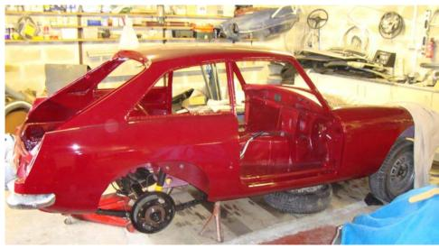
At long last I have the painted shell of Damask 450 back home in my garage. No doors, bonnet or tailgate at this stage. I have started the rebuild at the rear, fitting the leaf springs, rear axle, rear brakes and telescopic shock absorbers. There were a few problems:
