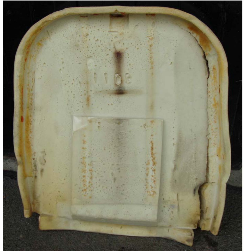
Photo (4) shows the back of an old seat foam. Note the square reinforcing panel. Unfortunately, without any added metal, this panel tends to slip between the bars. With my modification, it becomes a built-in lumbar support cushion.
