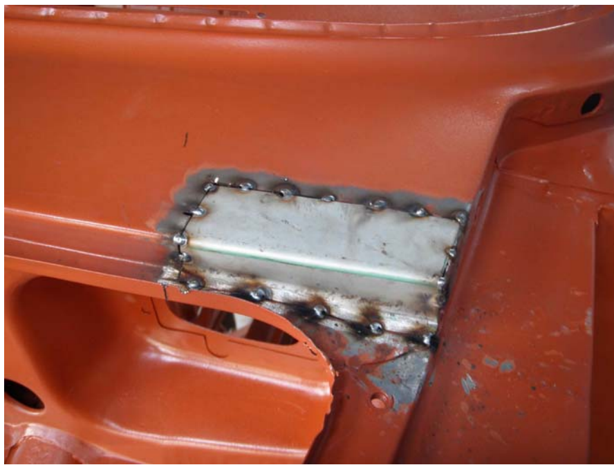
Above: metal panel welded in.
