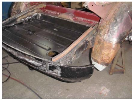
Inserting the boot floor was found to be easier with the whole of the rear bodywork removed from the shell. This also gave good access for welding the outer closure plates to the rear chassis extensions.
