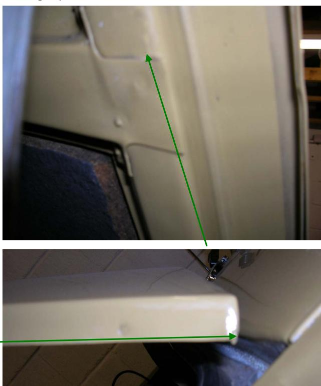
Measurement of the position of the cross brace on the underside of the bonnet from the nearside edge of the bonnet nearest the windscreen is **67.7cms** on an MGBGTV8. A similar measurement was made on the aluminium bonnet of an early MGB Roadster.
