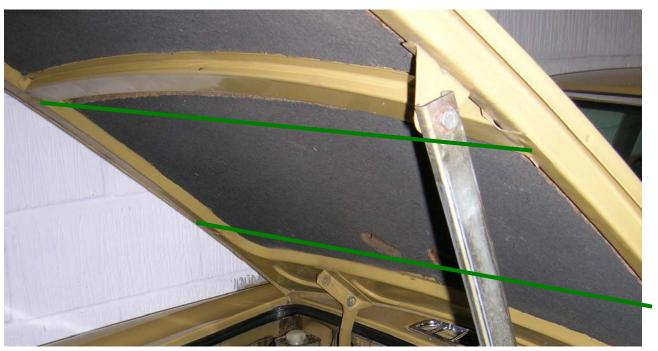
Measuring the profile/curvature of an MGB & MGBGTV8 bonnet
