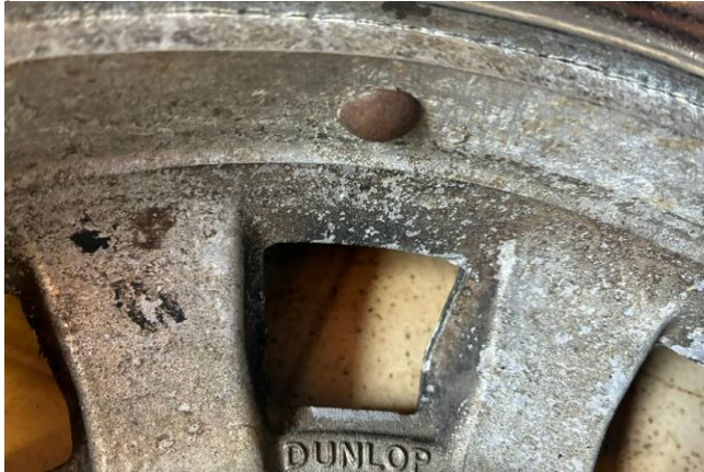
Cast aluminium centre is riveted to a rolled steel rim with iron rivets which create a galvanic corrosion risk
