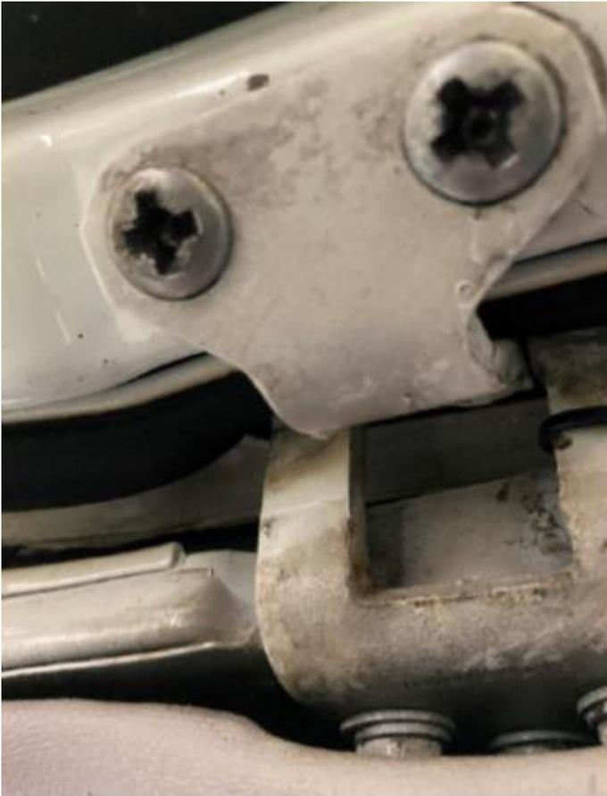
7. Using a PZ4 bit gradually loosen the four countersunk hinge screws.
