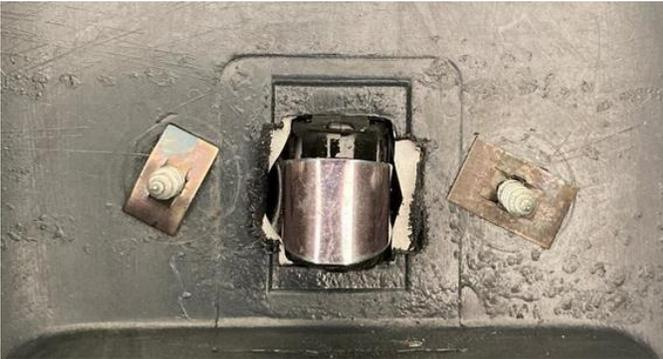
10. Remove the two screws holding the peg plate to the front underside of the armrest, remove the peg from the plate, refit at 90 degrees to its original position and reattach the assembly to the armrest.
