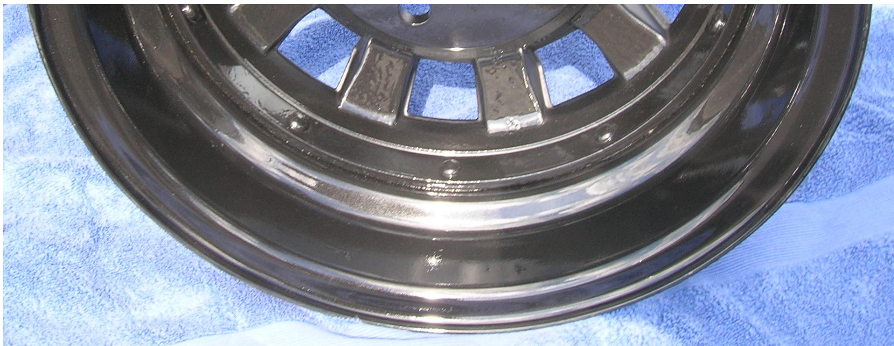
Above: silver top coat, lacquered with Polyurethane paint and a clear coat
