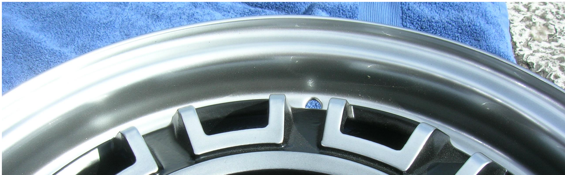
Above: silver top coat, lacquered with Polyurethane paint and a clear coat
