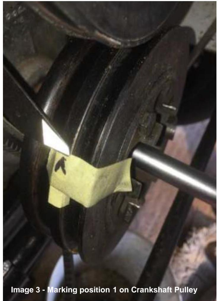
Image 3 - Marking position 1 on Crankshaft Pulley
