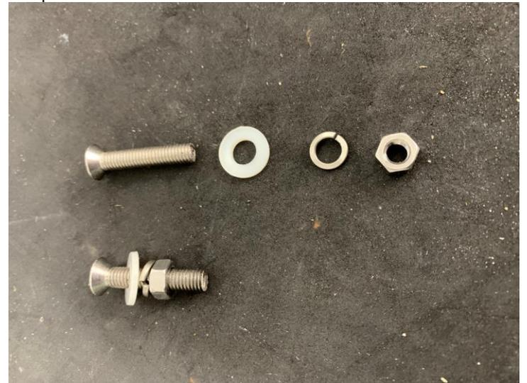
I then fitted the base plate into the two holes and placed the mounting plate over it. Two 25mm M5 countersunk machine screws were then threaded through the mounting plate to hold the parts in place. Fitting the plastic and spring washers and nuts onto the machine screws was technically simple but physically difficult. Without removing the window, the only access to the machine screw is
