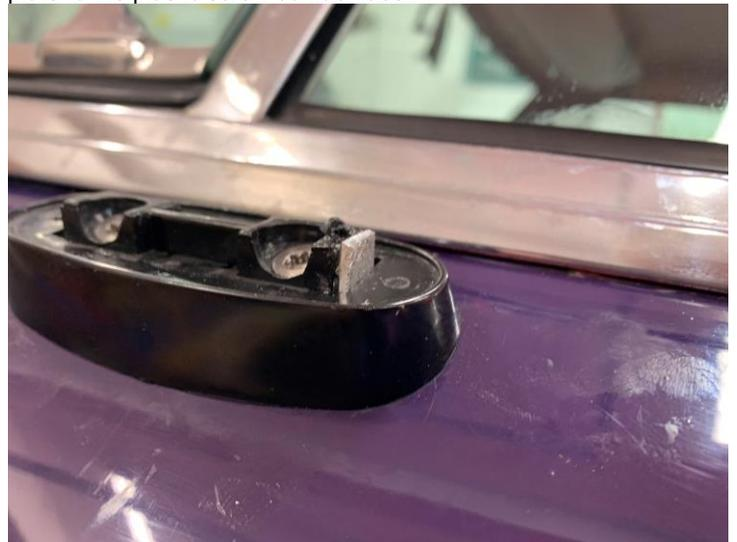
I then filed the base of the mirror to lower the point at which the grub screw contacts the plate. Sufficient material was removed to ensure the point on the grub screw contacted the middle of the aluminium plate and did not ride over the top.
