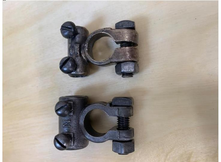
The original **earth lead** is mounted in the nearside cradle and merely needed to be cleaned (and shortened in my case, it was twice as long as necessary). Also clean the connection to the body to ensure a good earth in case any corrosion has built up
