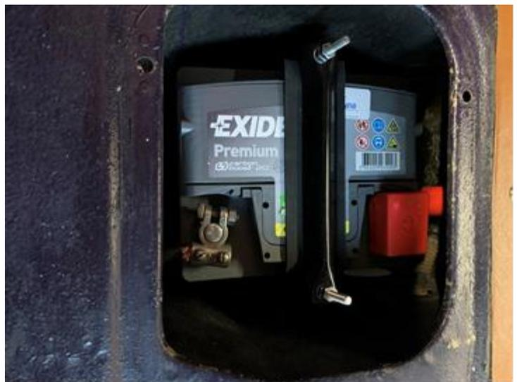
The retaining bracket normally fits across the end of the battery to accommodate the terminals. For this installation the bracket has to be fitted across the top. The 079TE is sufficiently tall that it is only necessary to shorten the threaded ends of the rods (the "J" peg battery holders) by about  $\frac{3}{4}$ " to avoid fouling the top access cover to
