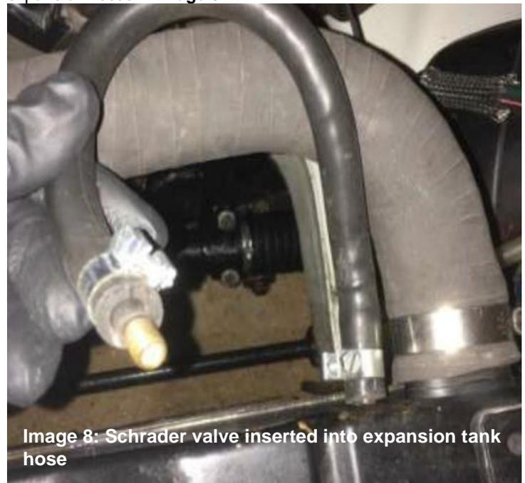
Image 8: Schrader valve inserted into expansion tank hose
