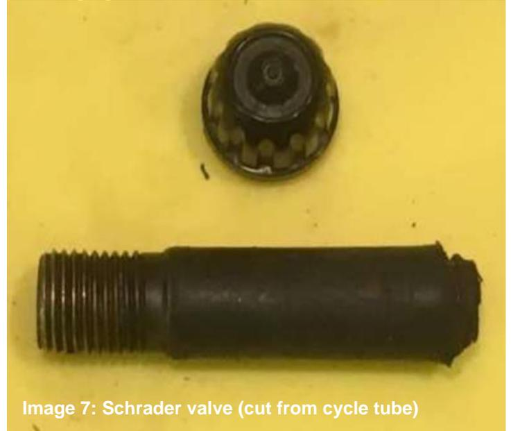
Image 7: Schrader valve (cut from cycle tube)
