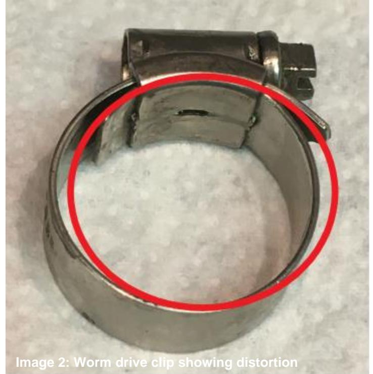
Image 2: Worm drive clip showing distortion
