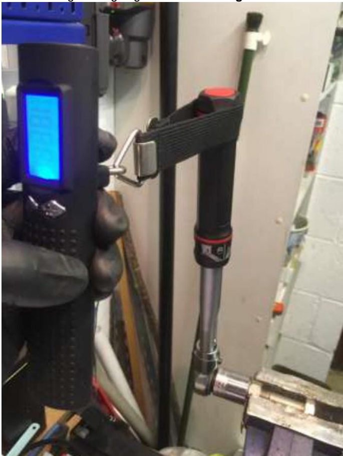
Image 9: Confirming calibration of torque wrench
