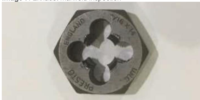
Image 8: 7/16" UNC die nut for bolt thread cleaning
