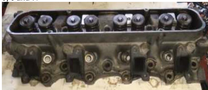
Image 6: Exhaust port inspection (note the leakage on cylinders 1 and 7)
