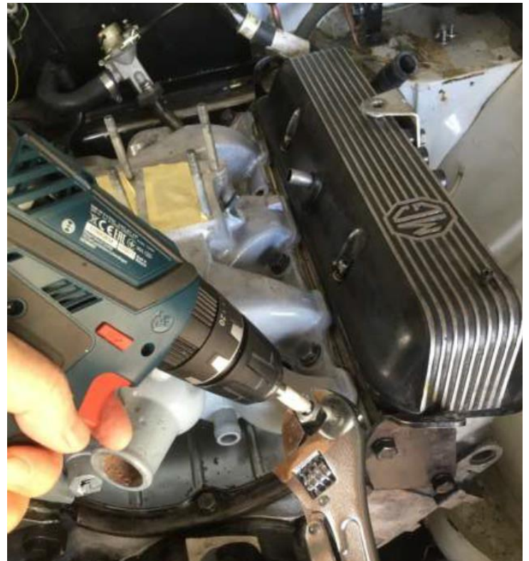
Image 7: Drilling through the bush (with wrench to prevent rotation)
