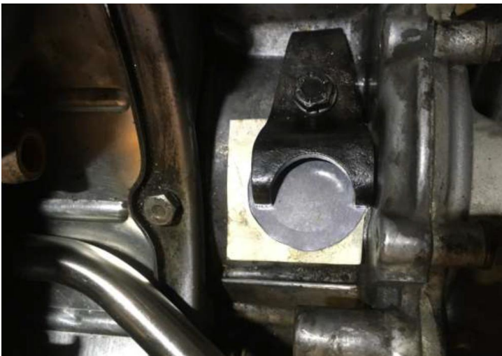
Image 5: Sealing the distributor aperture
