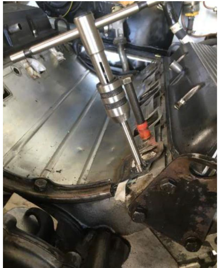
Image 11: Tapping for insert using guide bolt to aid alignment
