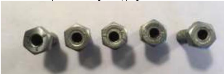
Drill bushes manufactured from 1/2" setscrews
