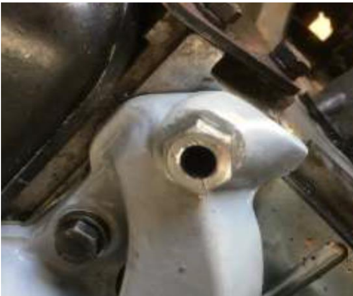
Drill bush in position in the inlet manifold
