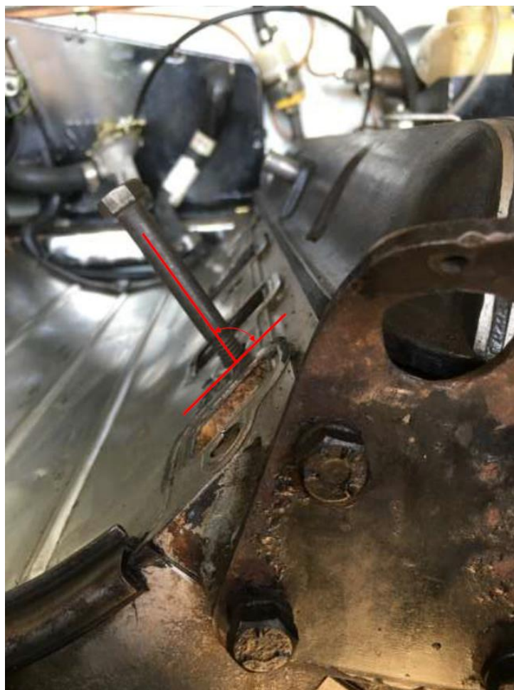
Image 2: Guide bolt demonstrating angle to joint face
