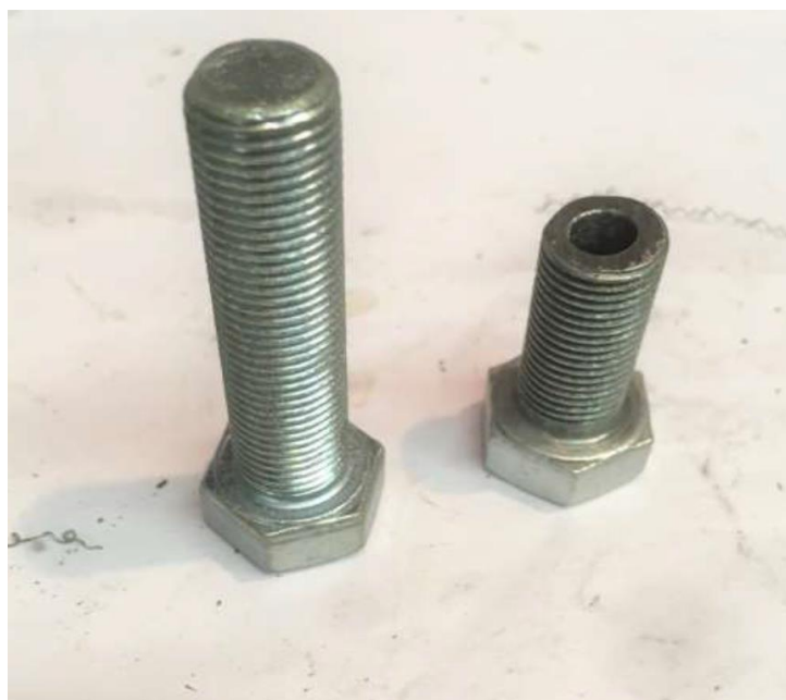
Image 3: Drill bush manufactured from ½" setscrew
