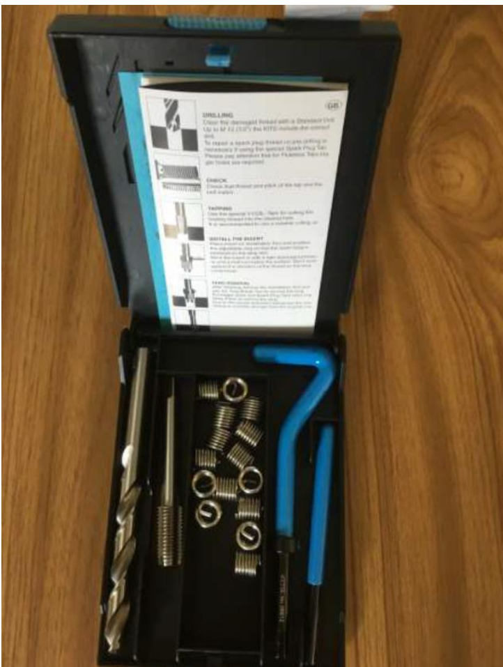
Image 10: Insert kit with (from left to right) drill, tap, inserts, insertion tool and tang break off tool
