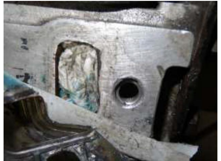
Wire thread insert installed
