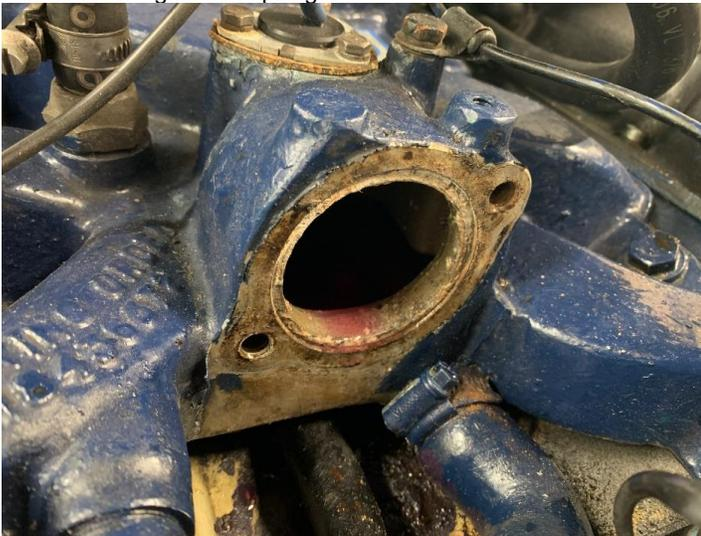
**Two hoses have to be removed** – the feed to the radiator and the “Steam Pipe, Thermostat to Manifold”. In this instance, the main hose had been replaced recently and came off easily. The Steam Pipe, however, could only be persuaded to part with the housing after the housing had been removed.
