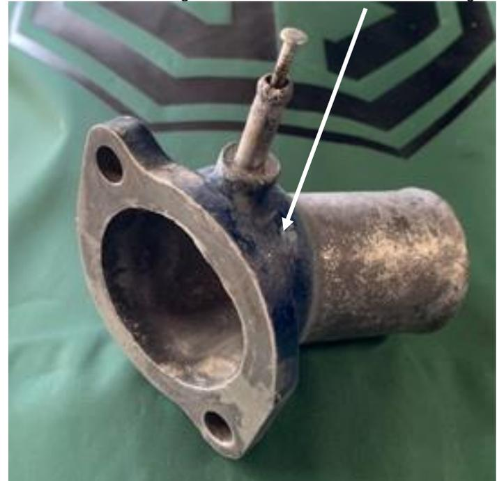
**Some cleaning was necessary around the manifold.** In addition to the removal of accumulated scale, a previous owner's blue brushed paint had to be paired back. Particular attention was paid to the shallow recess where the thermostat sits to ensure a good fit. It should also be noted that it is important to prevent ingress of contaminants into the cooling system.
