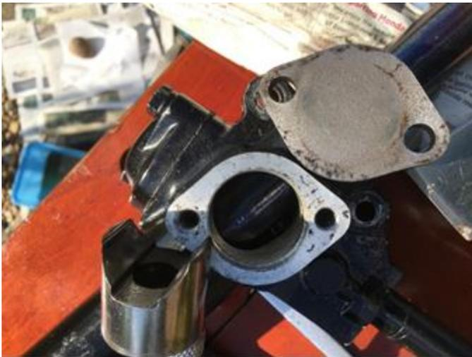
Image 8: rack damper housing with yoke and cover
