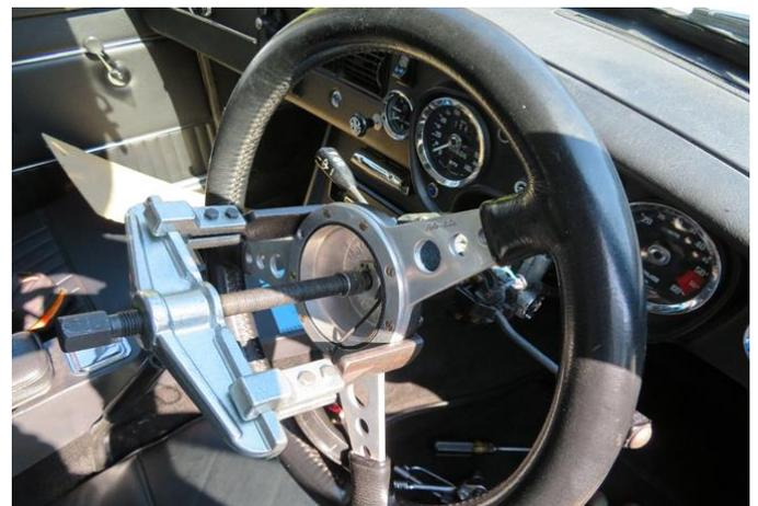
Image 2: removing the steering wheel
