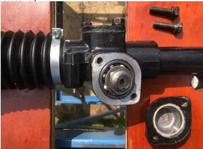
Image 4: pinion bearing housing and cover
