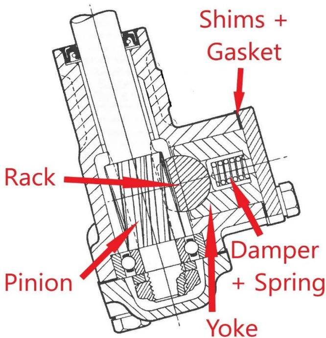
Image 7: rack & pinion sectioned view
