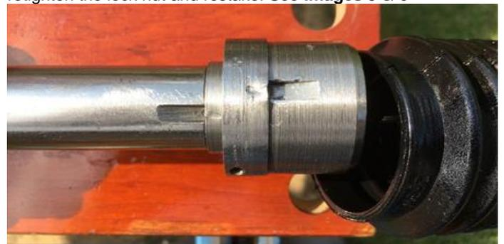
Image 6: rack inner ball joint showing staking
