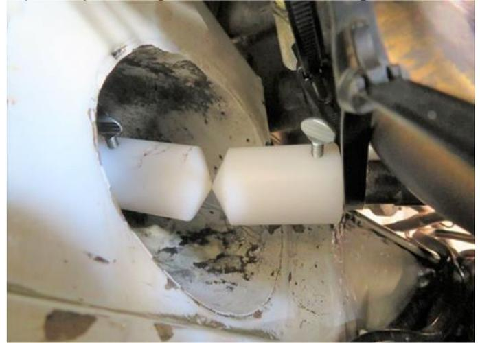
Image 9: aligning upper and lower shafts
