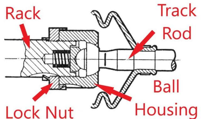
Image 5: rack inner ball joint sectioned view
