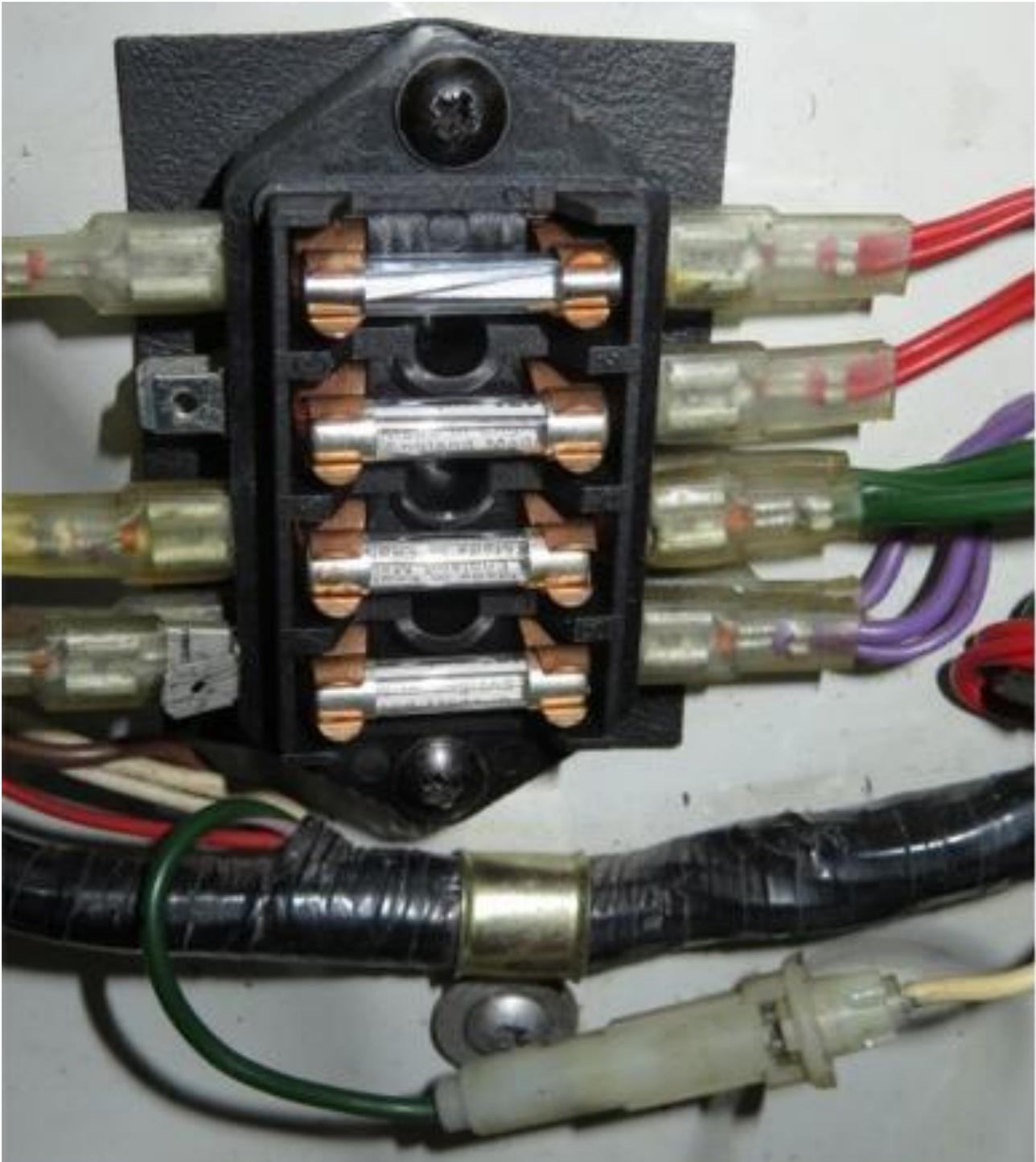
Completed fuse box installed on the offside inner wing.
