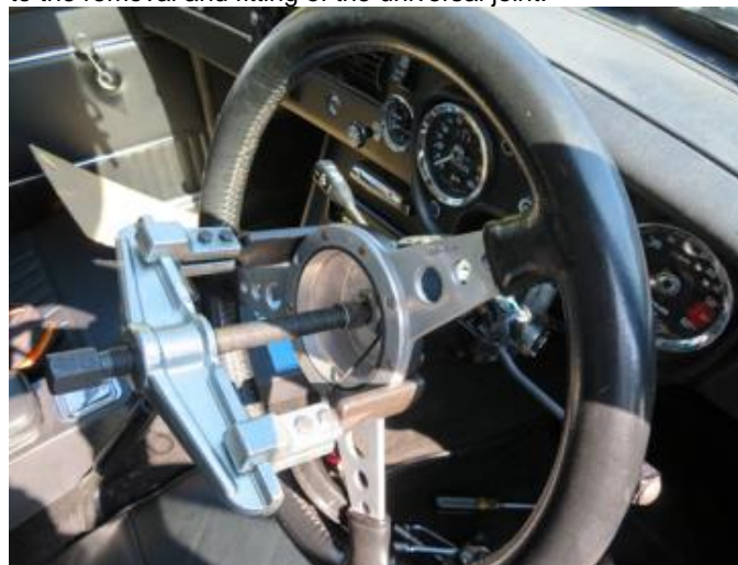
Image 3 – puller to remove the steering wheel safely
