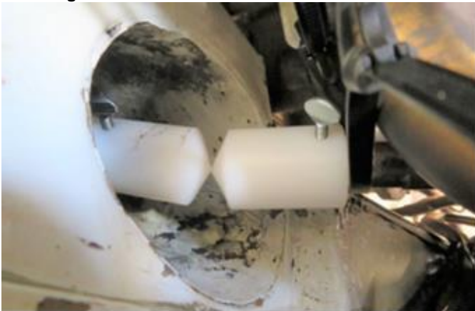
Image 10 – Aligning upper and lower shafts
