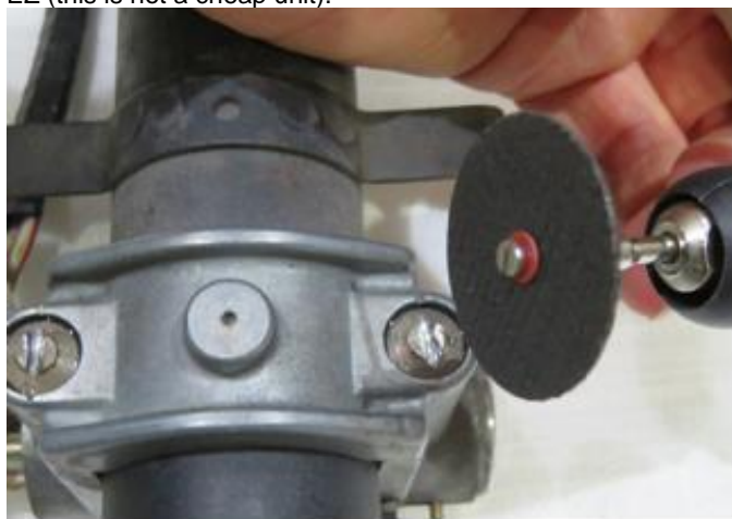
Image 5 – removing security bolts
