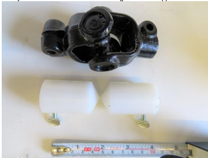
Image 2: - Column alignment tool
