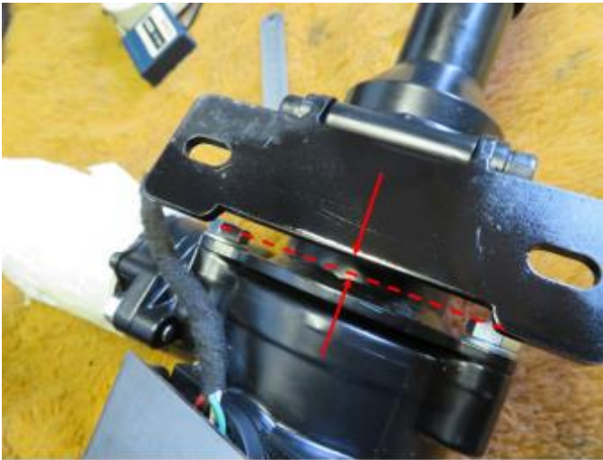
Image 9 – Lower bracket modification
