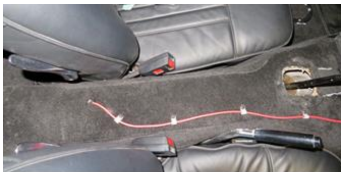
Image 15 – Power cable routing
