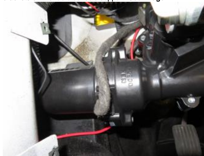
Image 7 – Motor unit in position
