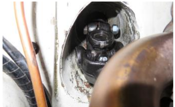
Image 13 – Upper universal joint bolt
