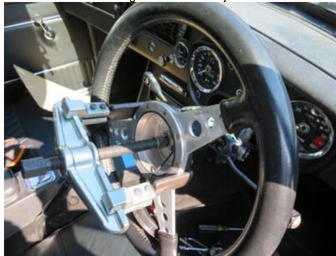
Image 3 – puller to remove the steering wheel safely
