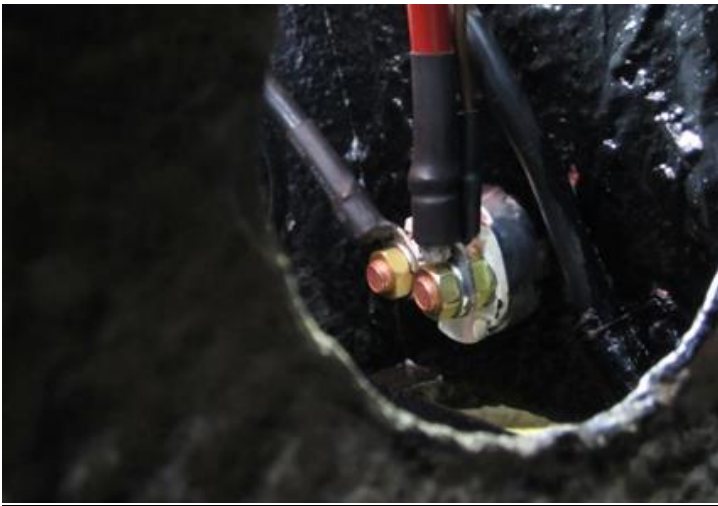
View through the opening in the right hand side of the battery box – Black cable originally connected to positive terminal of the battery now connects to the master switch. New red cable connects from the battery to switch.
