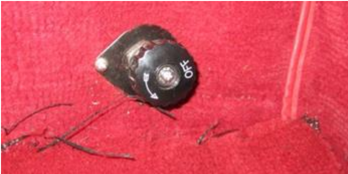
Durite Type 0-605-02 switch , which is a close copy of the Lucas Type SSB-103. A small black plastic disc is supplied to conceal the screwhead in the knob.
