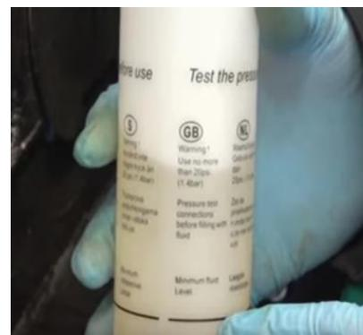
cylinder is automatically topped up by the Eezibleed kit. Continue bleeding until the fluid emerging runs clear and free of air bubbles. Then close off the nipple, taking care not to overtighten the nipple. Repeat on all the other brake nipples to complete the operation.
