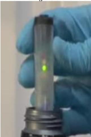
**Left:** the tester inserted in a container of new brake fluid shows a **green LED** which indicates there is zero water in the brake fluid. If you suspect the brake fluid may be contaminated with water simply insert the tester in the brake fluid reservoir – in the case **above right** the red LED shows there is water in there and the brake fluid needs changing.
