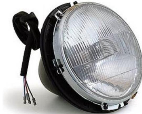
**Replacement 7” H4 Halogen headlamp unit** with main and dip beams with sidelight, metal reflector, plastic backshell, gasket and wiring harness. 'E' Marked. No Rim. Fitted with 12 volt Halogen bulb 60/65 watts and 5 watt sidelight bulb. Dips to the left hand side of the road.
