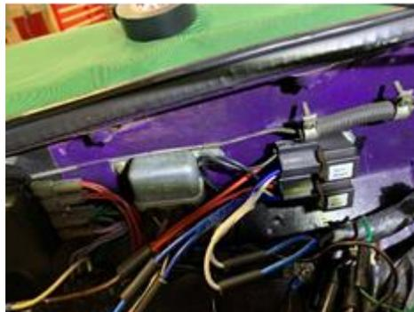
**Step 7 – Mount the relays.** Each of the relays has a mounting hole. Mark the centre of each on the offside inner wing and drill a hole appropriate to the size of the self-tapping screws to be used. Before mounting the relays, ensure that the bare metal resulting from drilling is adequately painted/protected. Mount the relays using self-tapping screws.
