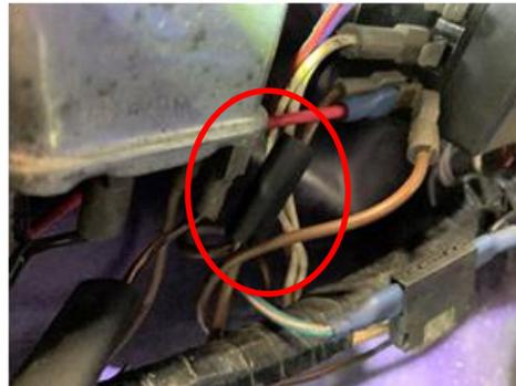
**Step 6 – Prepare the earth lead.** In this installation, the existing earth lead at the P clip securing the wiring loom near the relay is used. Clip the existing earth wire, add a bullet connector to each end and join with a double connector block.
