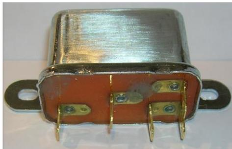
Original [6RA](#) relay fitted to the MGBGTV8
