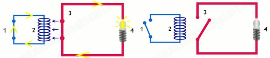
mechanical relays that work by activating an electromagnet to pull a set of contacts to make or break a circuit. These are used extensively throughout vehicle electrical systems and are useful where an in-line switch or the existing circuit does not have the capacity to handle the current required.
