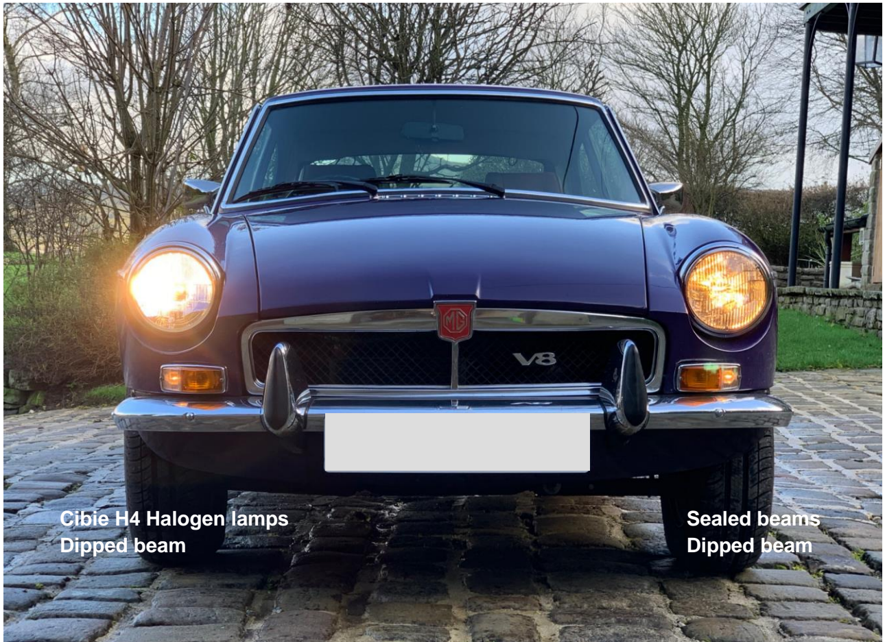
Cibie Halogen unit on the offside & sealed beam on the nearside, both on dipped beam . A most noticeable difference.
