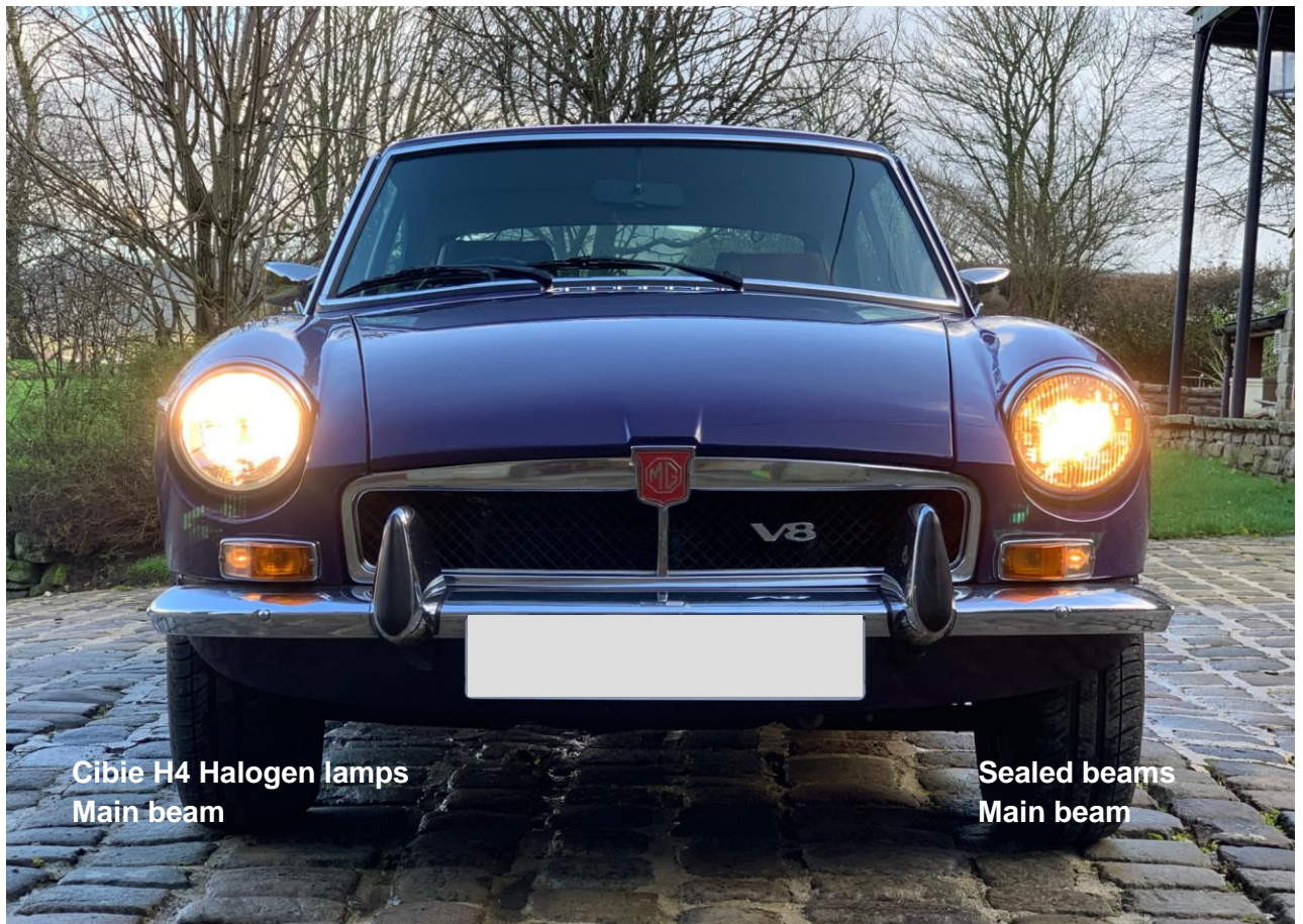
Cibie Halogen unit on the offside & sealed beam on the nearside, both on main beam . A major difference.
