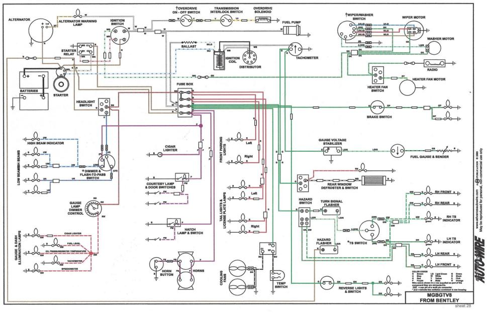
MGBGTV8 wiring diagram produced by Bentley (which in many respects is easier to follow than the diagram in the Driver's Handbook on page 46)
