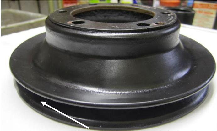
**Groove in the SD1 crankshaft pulley**
