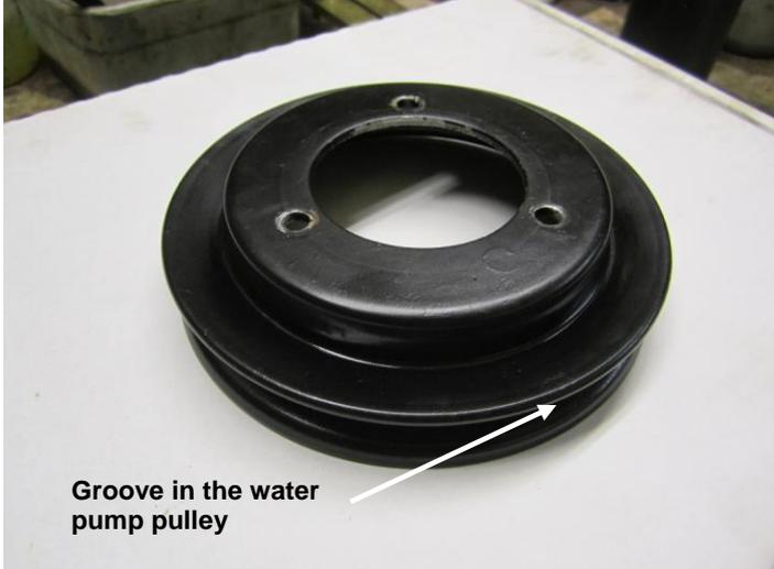
**Groove in the water pump pulley**
