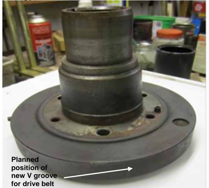
Planned position of new V groove for drive belt
