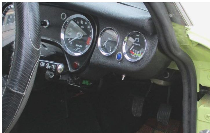
Push button located under the voltmeter in the dashboard.
