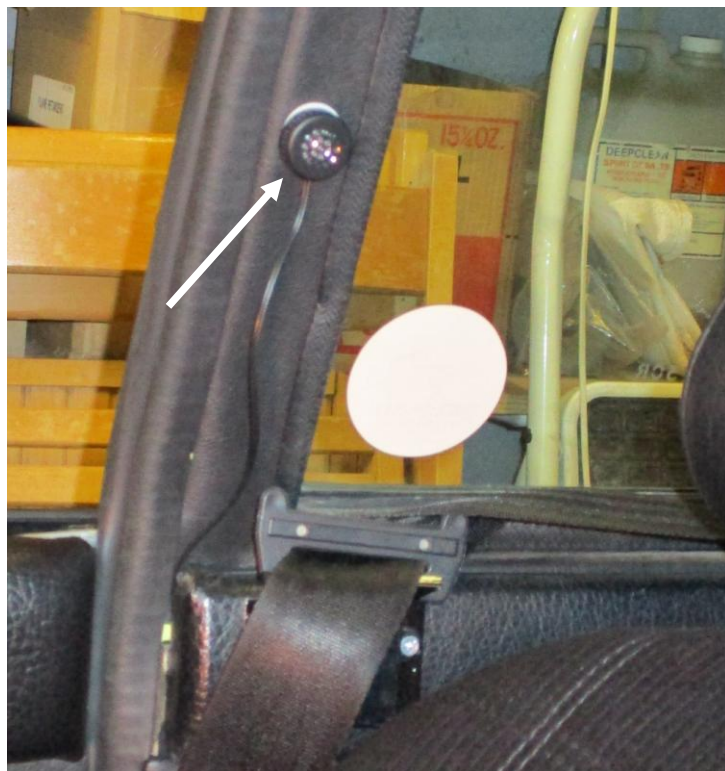
Buzzer is a small speaker half way up the pillar by the driver’s door.
